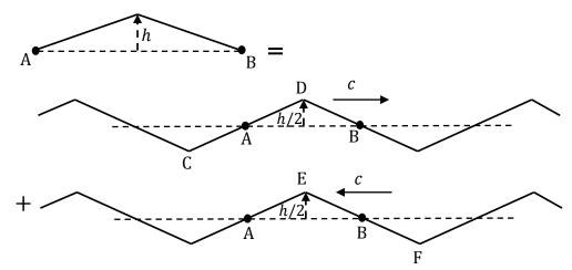
Both A and B will be fixed because two saw-tooth waves tend to move A or B in opposite directions. Clearly, the period of motion is the time for the saw-tooth wave to travel the distance 2*L*. Hence we obtain
