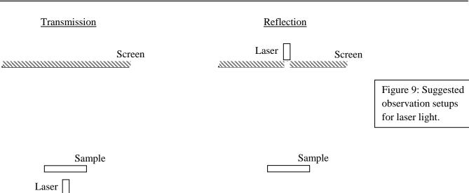
Observe the alternating pattern of bright and dim fringes on the screen as you slightly rotate the sample. The dimming of some of the fringes is due to destructive interference between different regions of each "tooth" on the sample.
