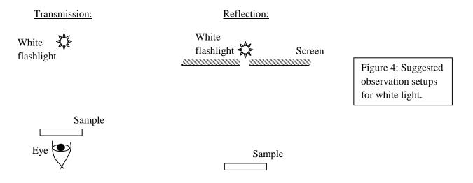
CAUTION: For viewing transmitted light, you will have to look directly into the flashlight beam through the sample. **Don't do this with the laser!** Also, avoid looking directly into the flashlight itself for long periods of time.
