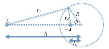
Figure 3: Two line charges with its equipotential surfaces
