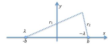
Figure 1: System with two line charges
