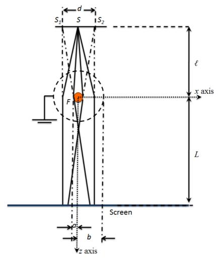
The electron "biprism" consists of a grounded cylindrical wire mesh with a fine filament F at the center. The distance between the source and the "biprism" is  $\ell$ , and the distance between the distance between the "biprism" and the screen is L.
